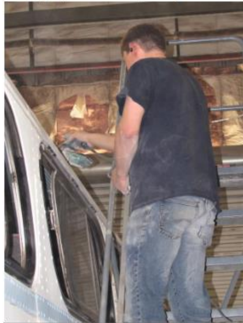
Tyler Johnson sanding the roof for painting Andy Goddard photo
