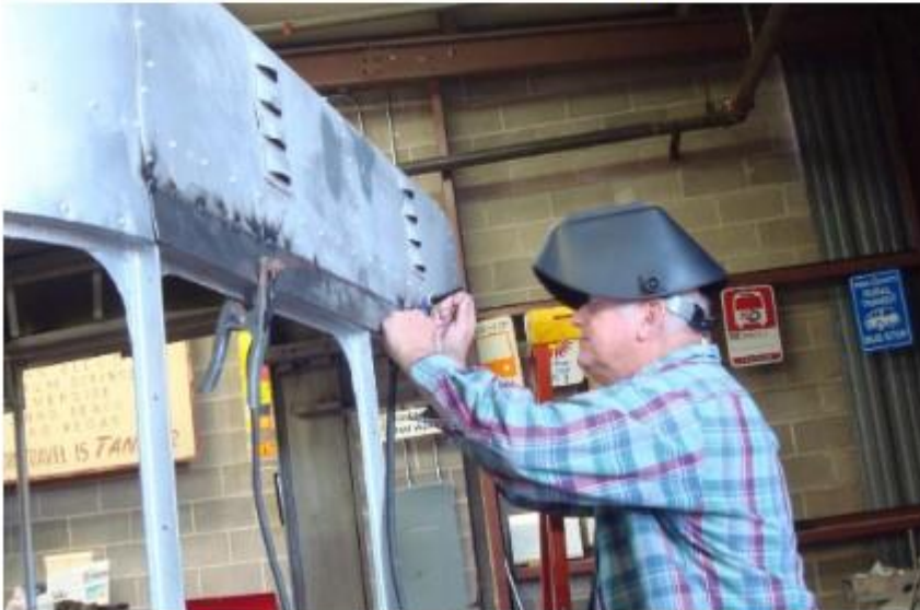
Dave welding new strip on rear of the 1928 Twin Coach replacing a badly rusted section on 12/20/10
